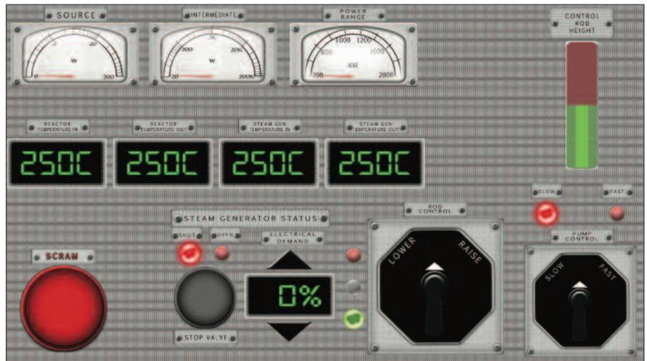
From the control panel of the Drexel simulator, users can control criticality, cooling, and electrical demand.
