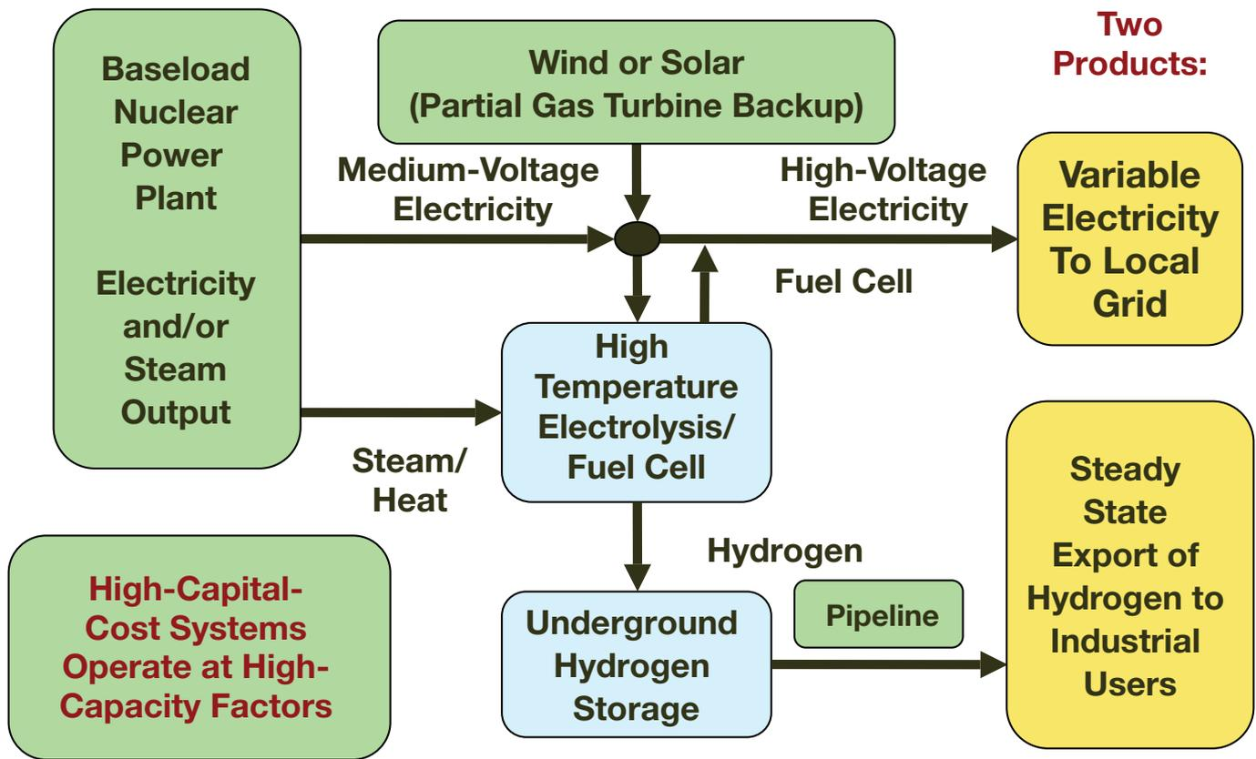
**Fig. 3.** Electricity-hydrogen system design
