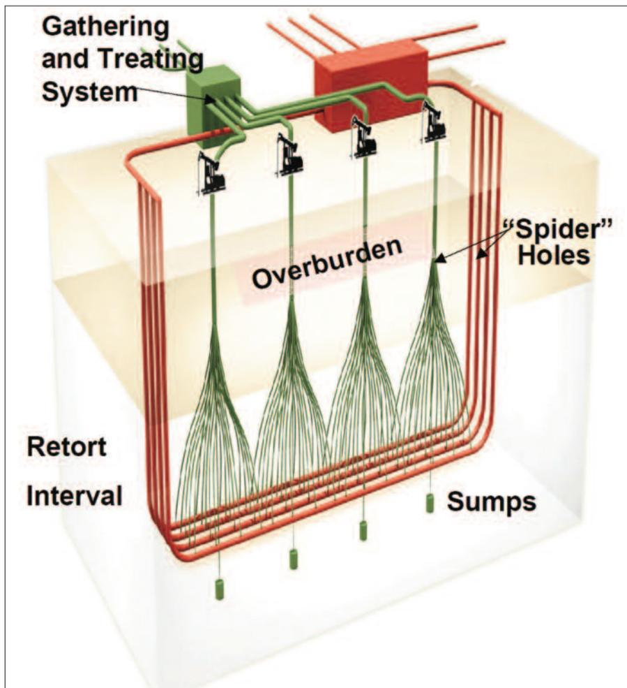
**Fig. 1.** Conceptual diagram of nuclear-geothermal energy storage system
