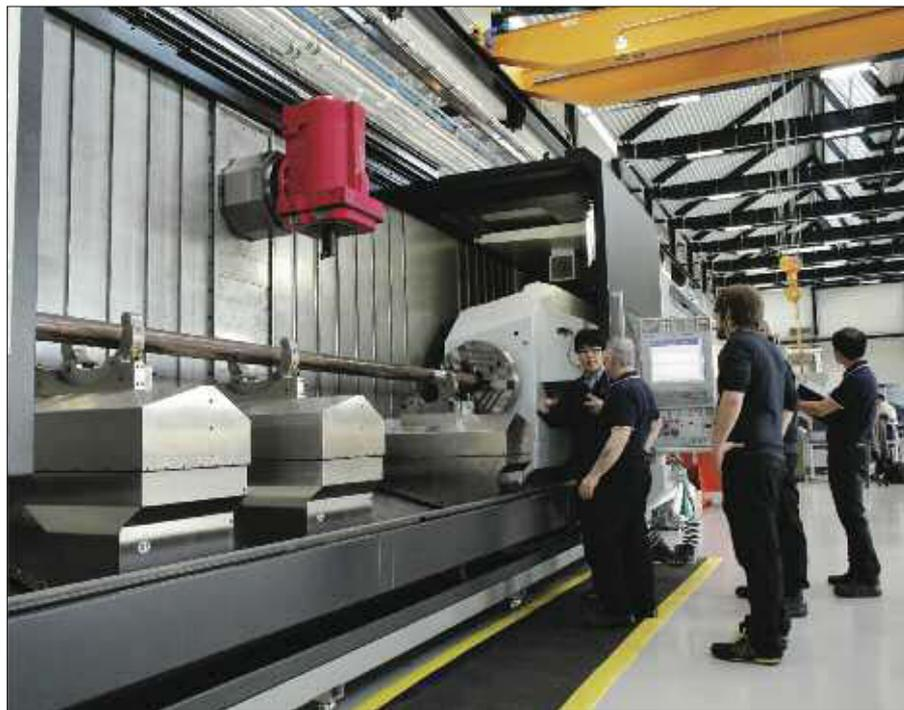
A Mori Seiki NT600 high-precision, high-efficiency integrated mill turn center is used for machining precision parts at the Nuclear AMRC.
