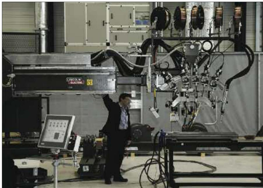
With advanced equipment such as the large-scale submerged arc welding station shown above, promising innovative welding techniques developed at the University of Manchester's laboratories will be able to progress to production readiness at the Nuclear AMRC.
