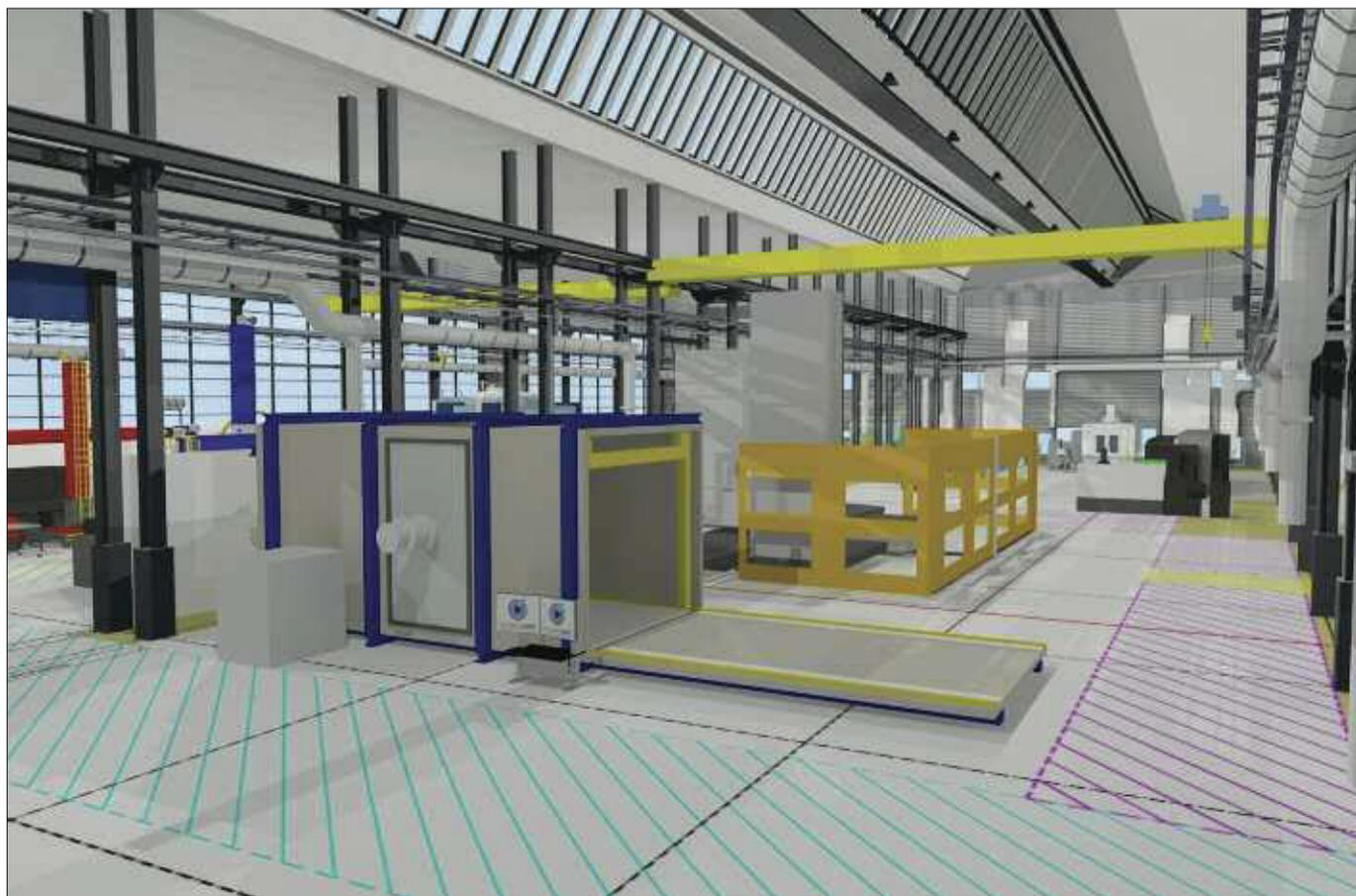
A computer-generated image of the electron beam welding chamber, which will be used to develop innovative joining techniques for large components such as pressure vessels. (Graphic/photos: Nuclear AMRC)
