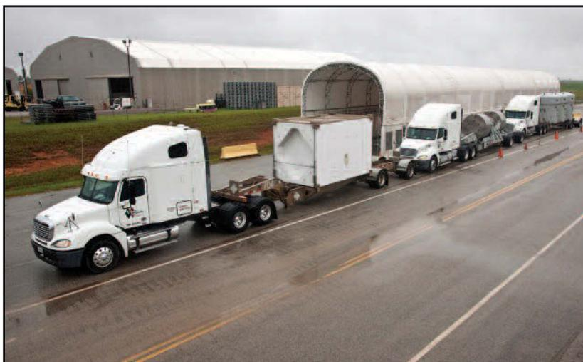
Three trucks, each bearing a different type of TRU waste container, get ready to leave the Savannah River Site, heading for the Waste Isolation Pilot Plant in New Mexico.
