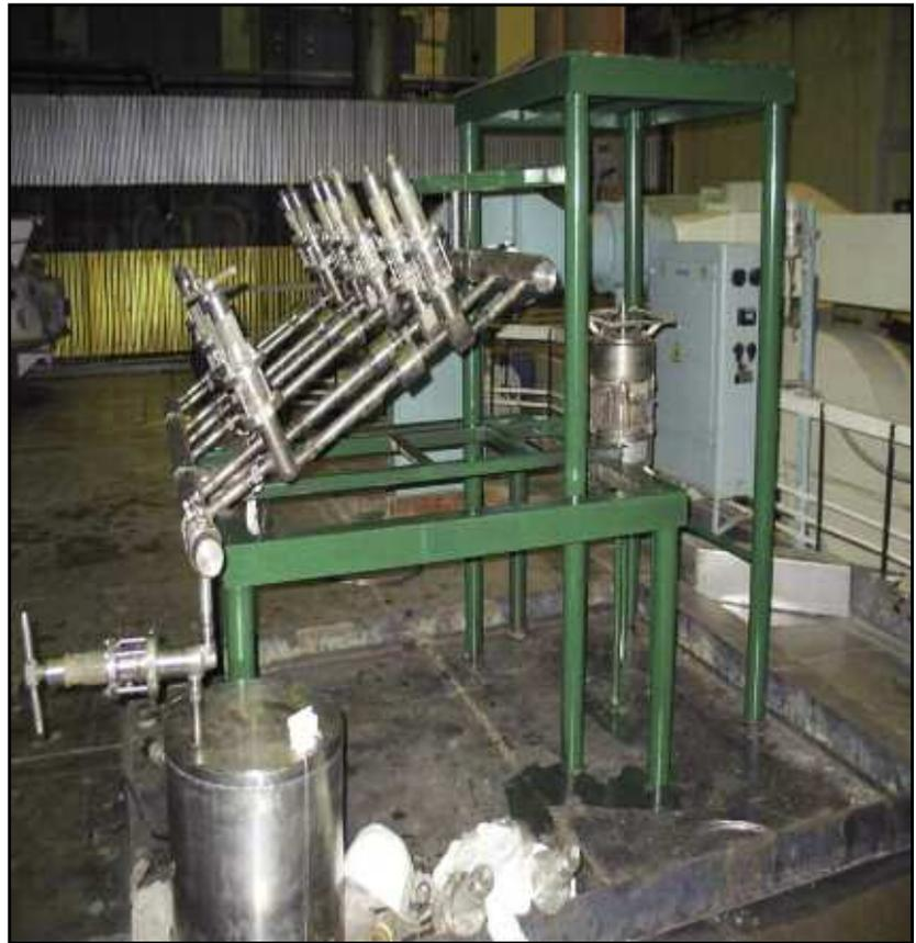
*Cesium Trap lead filling test rig.*
