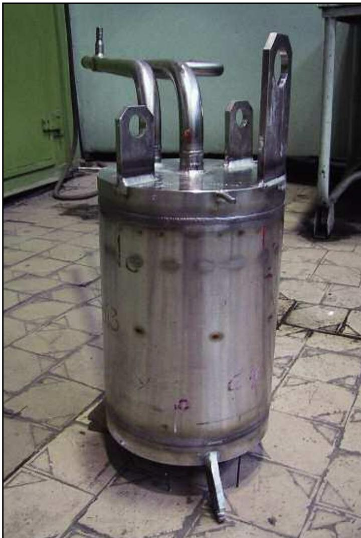
*U.S.-Kazakhstan design cesium trap (shown without shielding).*
