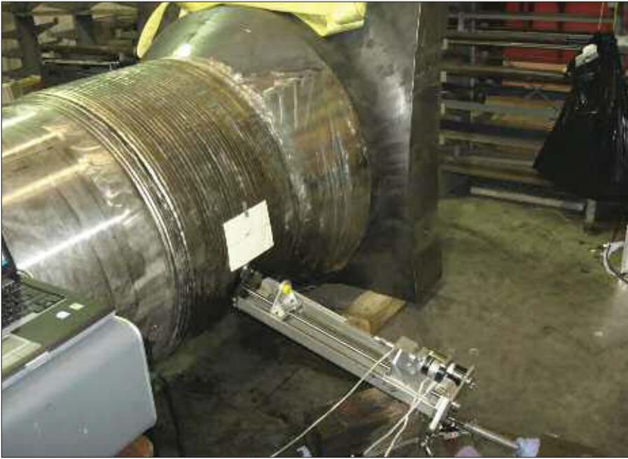
Measuring residual stresses through a mock-up of a cold-leg nozzle with weld overlay
