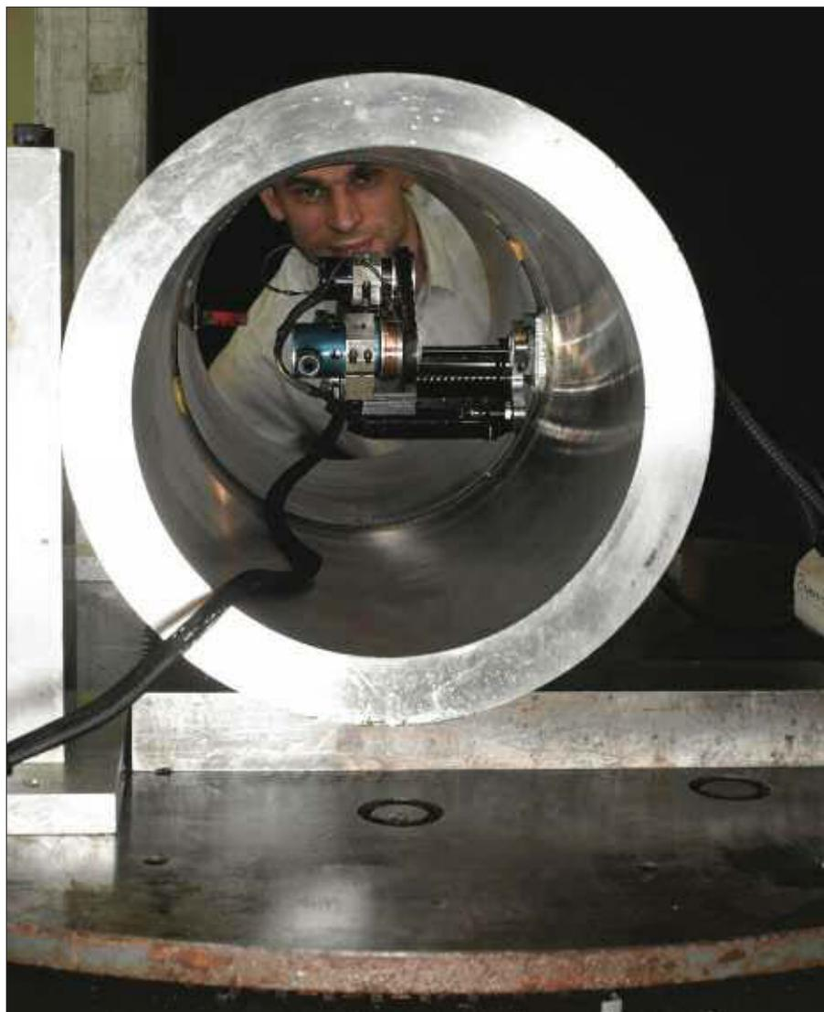
The mini deep-hole drilling machine was developed for measuring residual stresses from the internal diameter of a pipe in cases where the external diameter is difficult to access.
