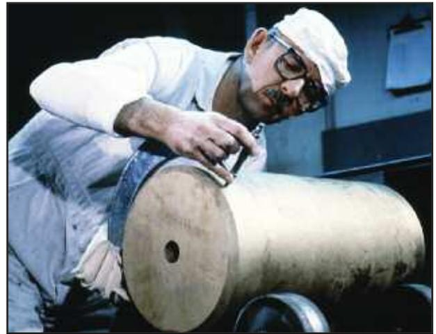
When "feed" materials left Fernald, they were in the form of finished fuel cores or cylindrical billets, which were re-shaped or finished at other DOE sites.
