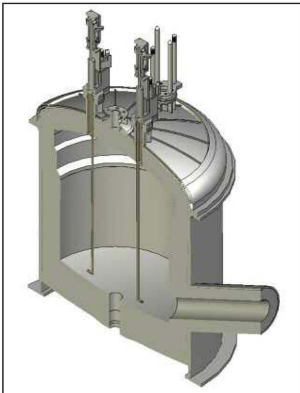
*Cutaway drawing of DWPF melter with two bubblers inserted.*
