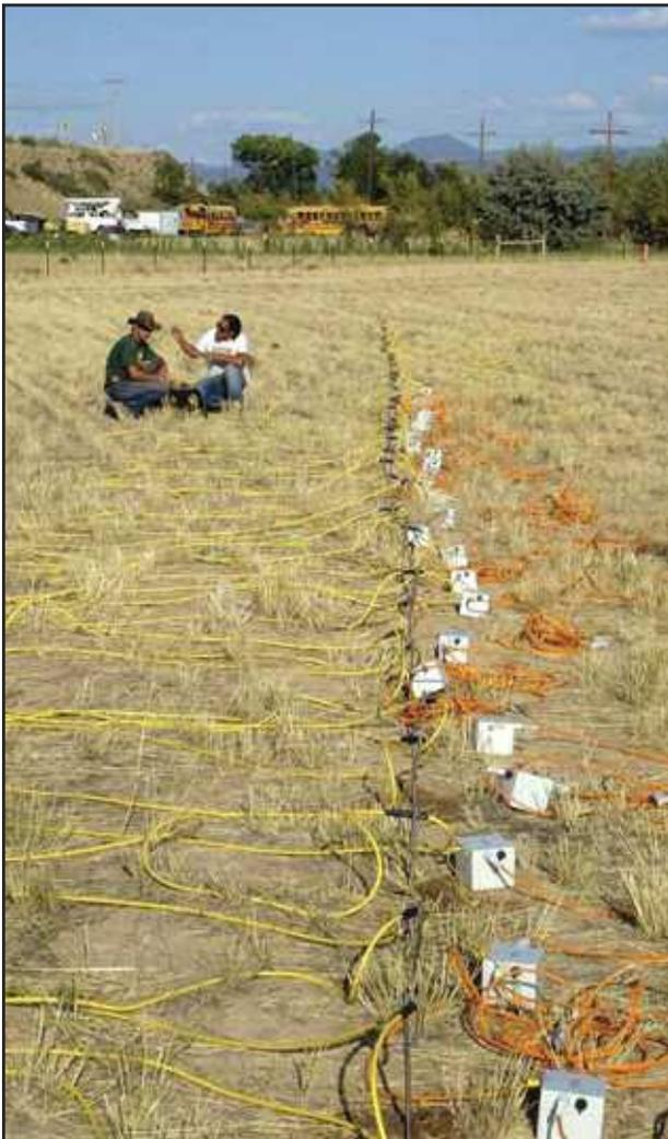
**Left:** Kenneth Williams, of Berkeley Lab, and graduate student Adrian Flores Orozco, of the University of Bonn, collect surface spectral-induced polarization at the Rifle Integrated Field Research Challenge Site. This work is helping to detect and delineate regions of naturally elevated subsurface microbial activity that could aid in halting the progress of radionuclides and other contaminants.
