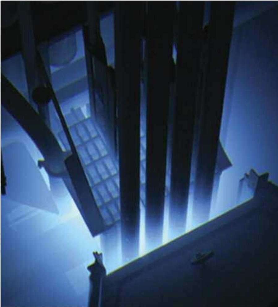
A view of the core of the PULSTAR reactor at 1-MW
