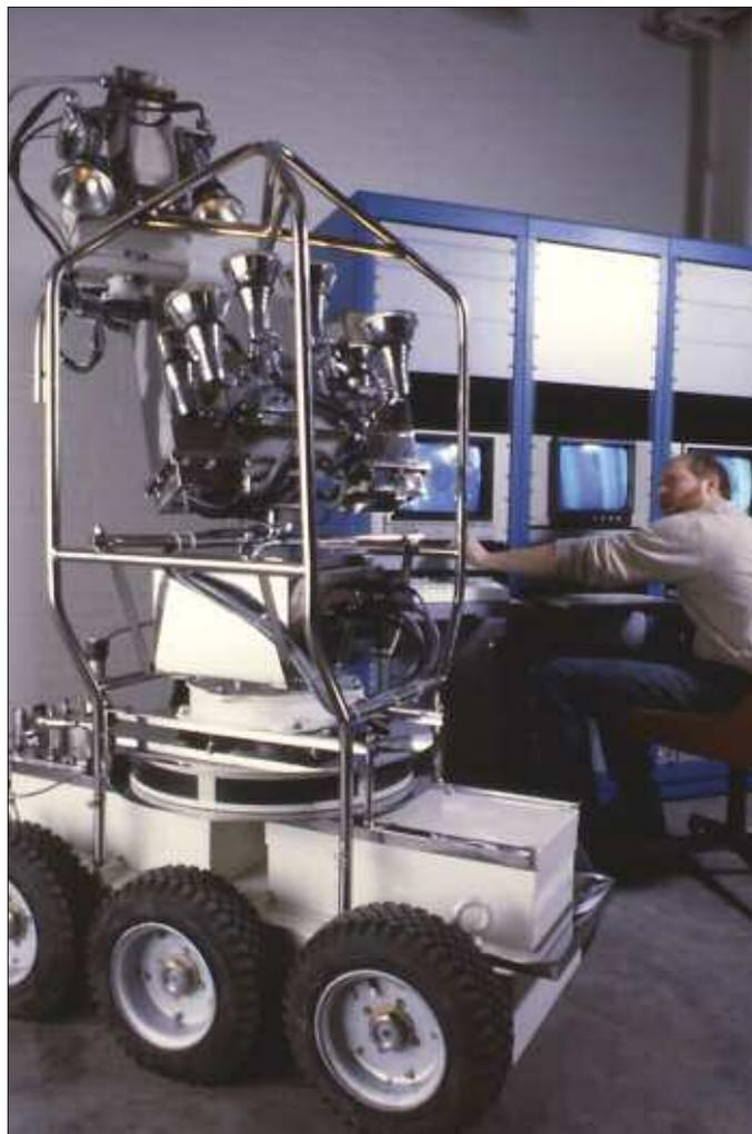
The Remote Reconnaissance Vehicle characterized the basement at TMI-2 and then went on to perform most of the robotic cleanup work. In the background, Red Whittaker sits at the control console in the operator station. (Photos: Carnegie Mellon)
