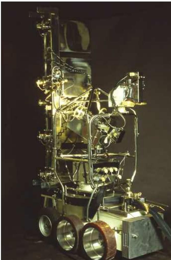
The Core Sampler extracted samples from TMI-2's basement walls. From these samples, the depth and severity of contamination was determined at several heights.
