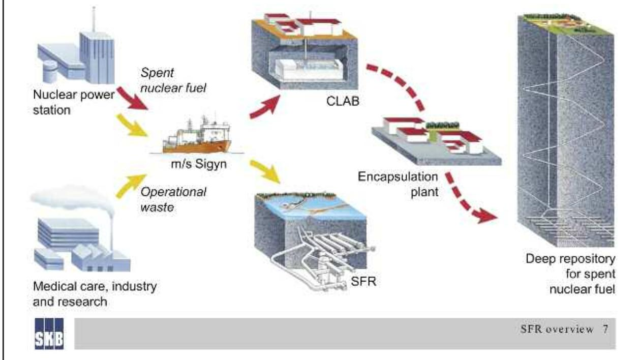
Fig. 1. Schematic illustration of core components of the Swedish nuclear waste management and disposal program/system. (Illustration courtesy of SKB.)
