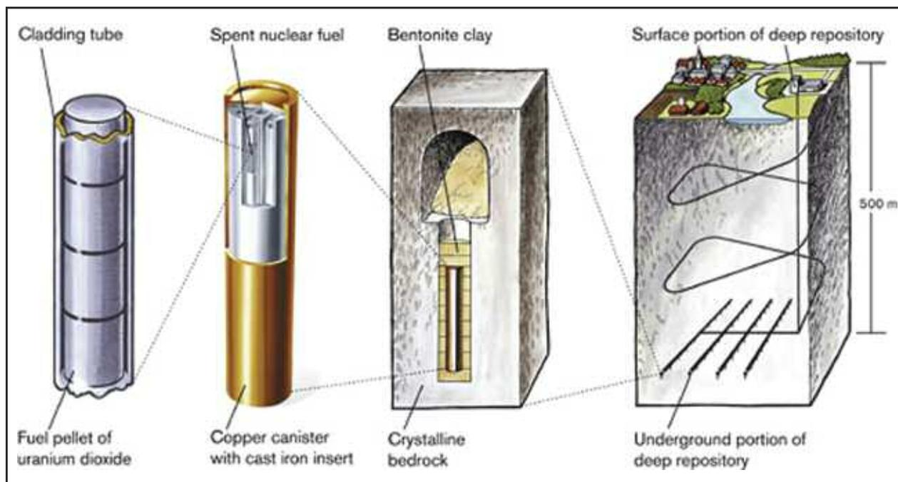
Fig. 4. Schematic illustration of the Swedish SKB-3V disposal concept (500 m = ~ 1640 ft). (Illustration courtesy of SKB.)
