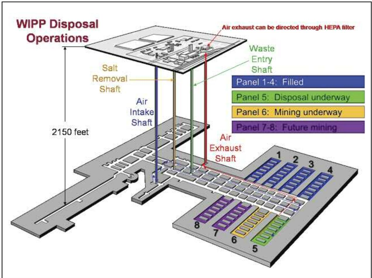
Fig. 2. Schematic illustration of the layout and current status of the WIPP transuranic waste repository. (The tunnels left of the air exhaust shaft, also referred to as the North Experimental Area, have been used since the late 1970s for full-scale transuranic waste, spent fuel, and HLW tests.)
