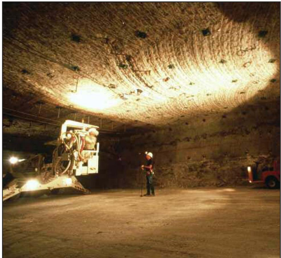
*Roof bolting allows rooms to be maintained open and safe for as long as needed to complete emplacement operations.*
