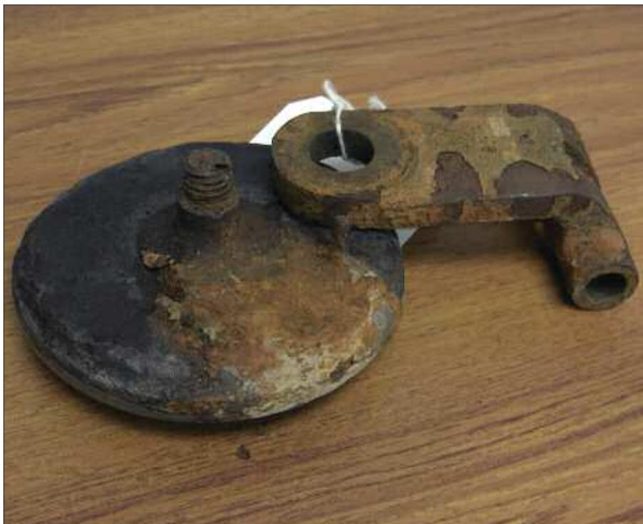
Check valve parts with the condition code "E," for "extremely degraded"
