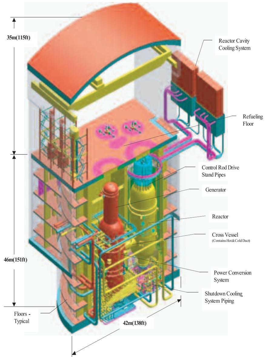
The MHR design features passive safety, deep-burn fuel, and high thermal efficiency. (Illustration: General Atomics)
