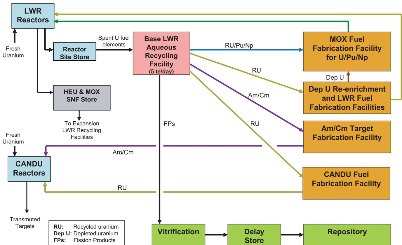
The flowchart shows the EnergySolutions team's short-term plan for recycling spent fuel before ARRs are built and brought into operation. In this plan, which includes americium and curium separation, technology demonstrations would start right away to support LWR aqueous recycling operations in the 2023–2035 time frame without the use of ARRs. The plan would be dependent on successful completion of the development of a separations process and of target manufacture. (Chart: EnergySolutions)
