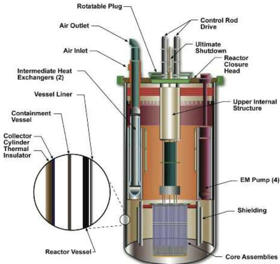
The internals of the GE-Hitachi team's PRISM reactor (Illustration: GE-Hitachi)
