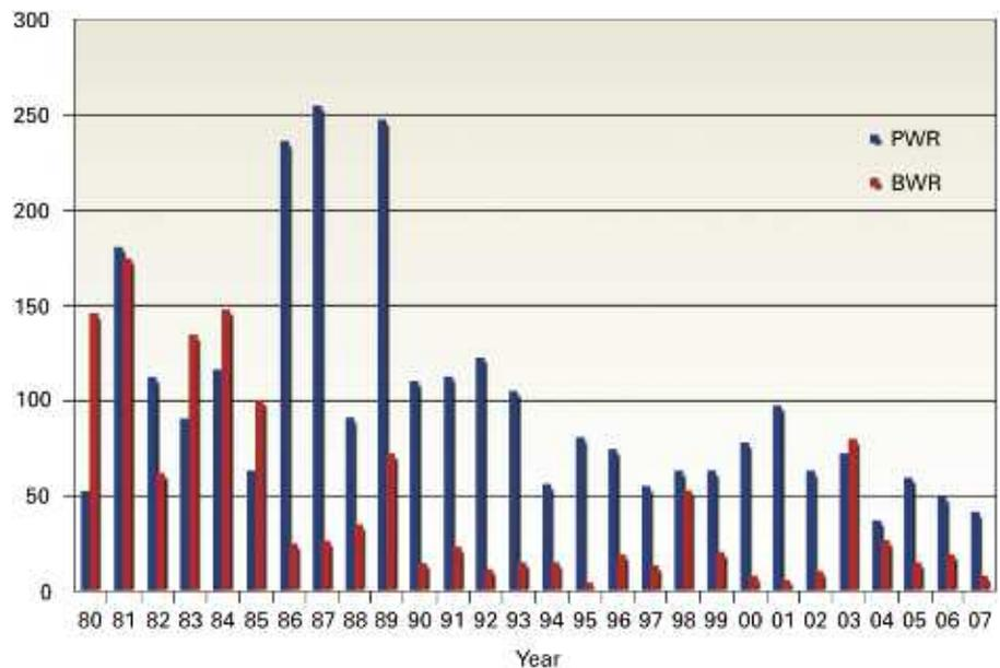
Fuel failures in U.S. PWRs and BWRs, 1980–2007 (Graphics: EPRI)
