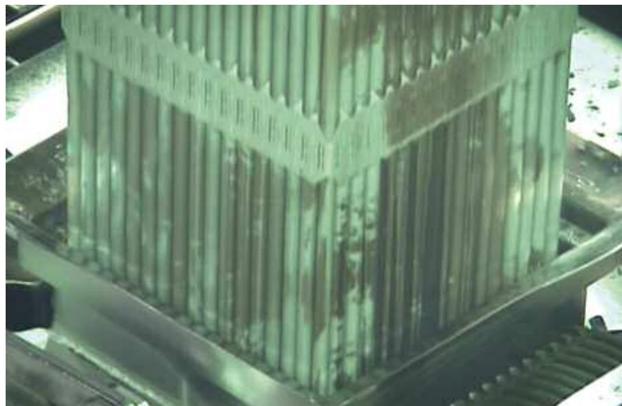
Visual inspection of a fuel assembly to assess crud loading
