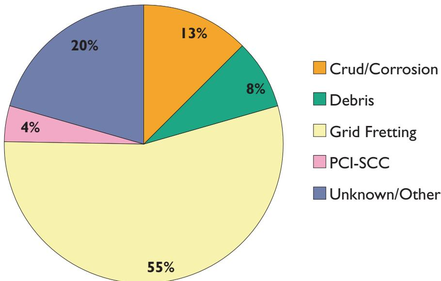
Percentage of fuel failures by mechanism for PWRs and BWRs, 2000–2007
