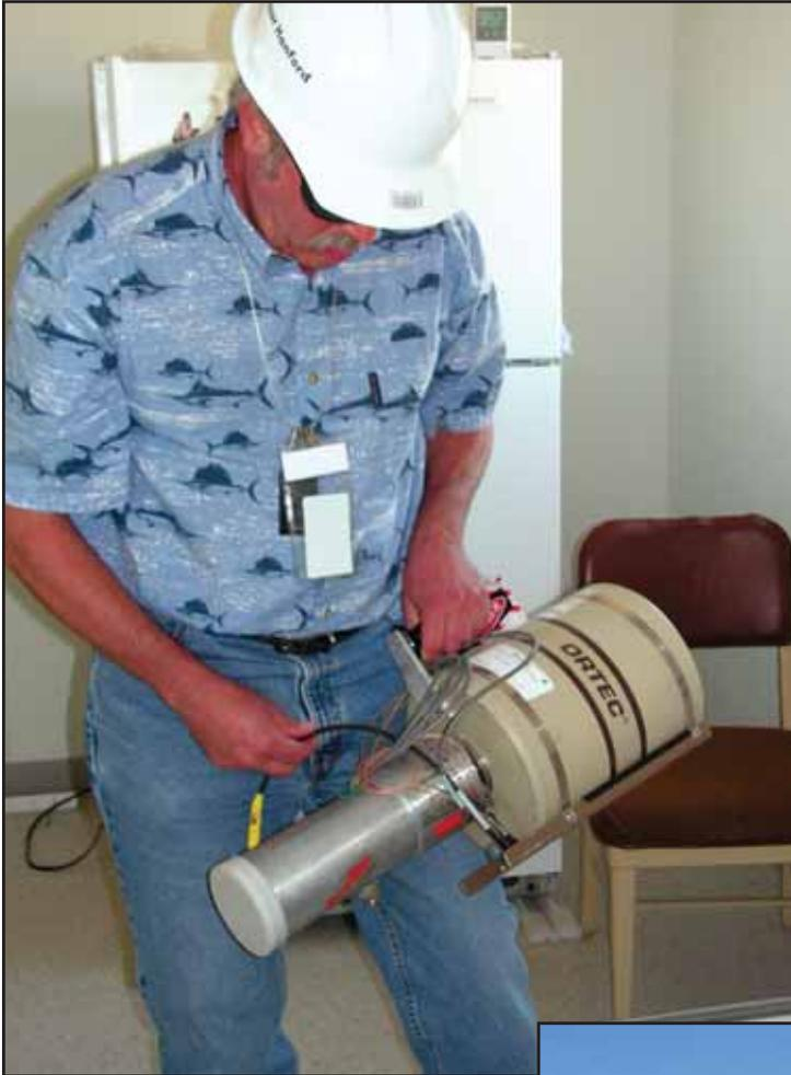
Jeff Pappin, Fluor Hanford Radiation Protection, Soil and Groundwater Remediation Project, displays one of many radiation-detection instruments acquired by Hanford from Fernald. This “GeLi” detector can analyze a multichannel spectrum to identify radioactive isotopes.
