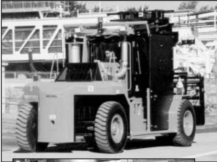
**Photos on Left: Top:** This 50 000-lb-capacity forklift truck was specially designed to transport heavy waste boxes for processing through the RHWF.
