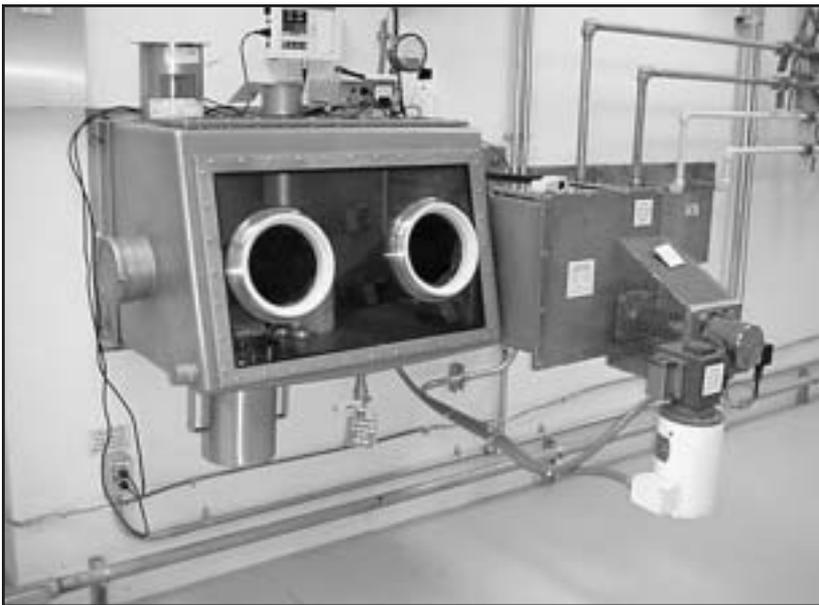
*This glovebox will allow operators to safely handle samples of material from waste boxes being processed through the facility.*
