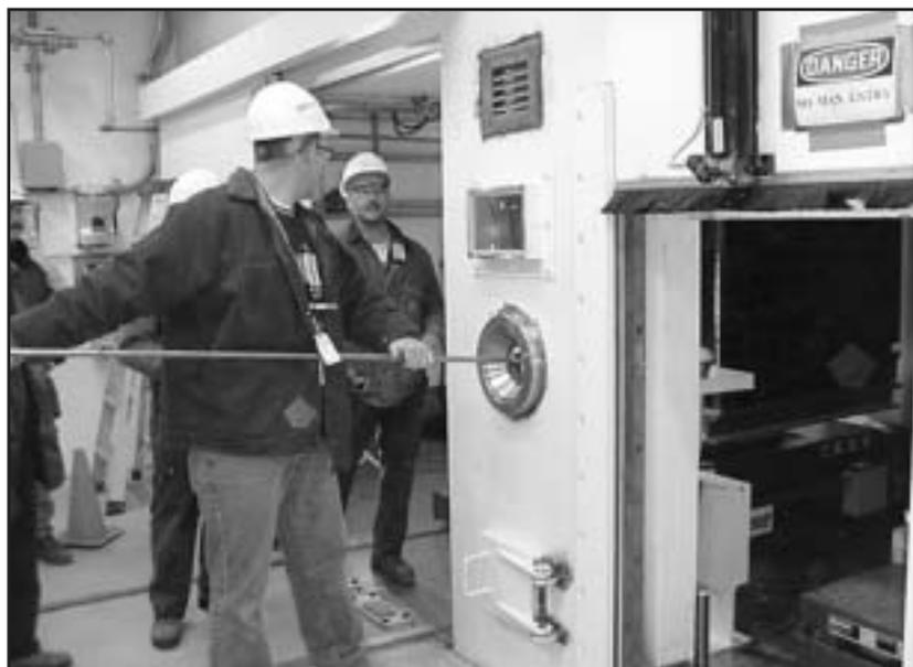
*Operators practice manipulating a reach rod during testing operations to take smear samples of boxes and drums in the waste packaging area.*
