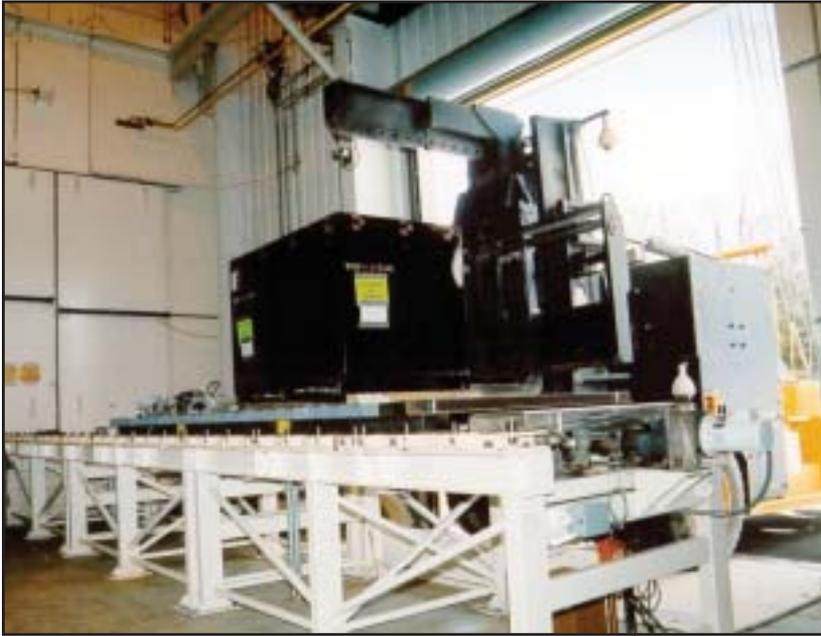
A mock box of waste is placed on the facility's roller system during testing operations.
