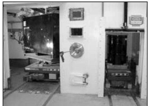
*The waste packaging system allows for bagless transfer of wastes from boxes and drums through these ports, shown during testing.*
