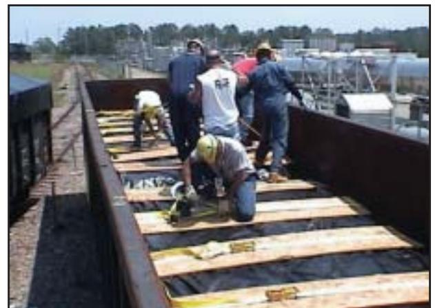
*Teams securing tie-down straps for loaded drums of depleted uranium oxide from the SRS, prior to shipment in gondola railcars.*
