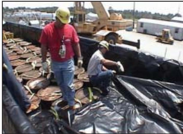
*Drums of depleted uranium oxide from the SRS being covered with liner after being loaded into gondola railcars.*
