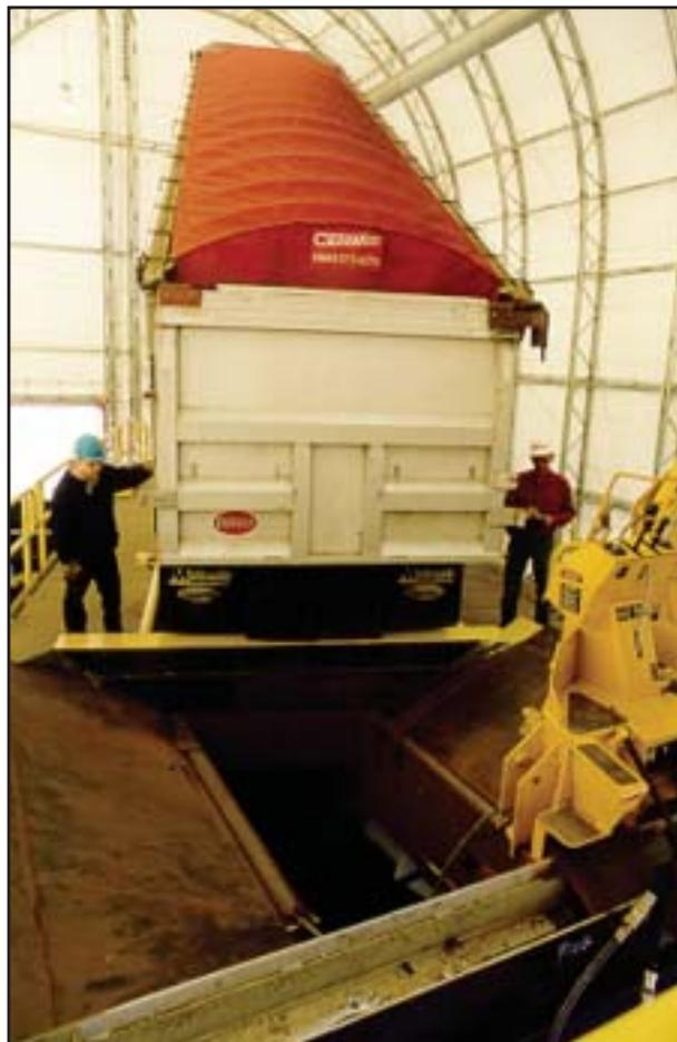
*Bulk materials inside MHF Logistical Solutions' totally enclosed transload facility in Worcester, Mass., being transloaded from a truck to a gondola railcar, positioned below, for shipment by rail.*
