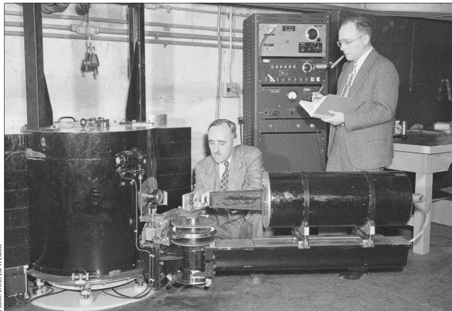
Ernest Wollan and Clifford Shull with their double-crystal neutron spectrometer at the face of the Graphite Reactor in 1949.
