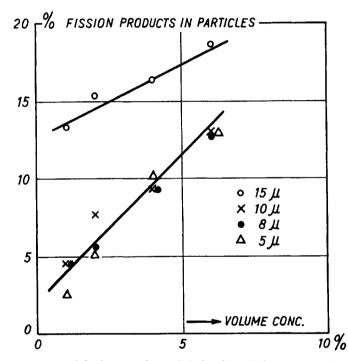
FIG. 1. The percentage of fission products left in the solid as a function of the volume concentration of uranium dioxide suspensions of different particle sizes.
