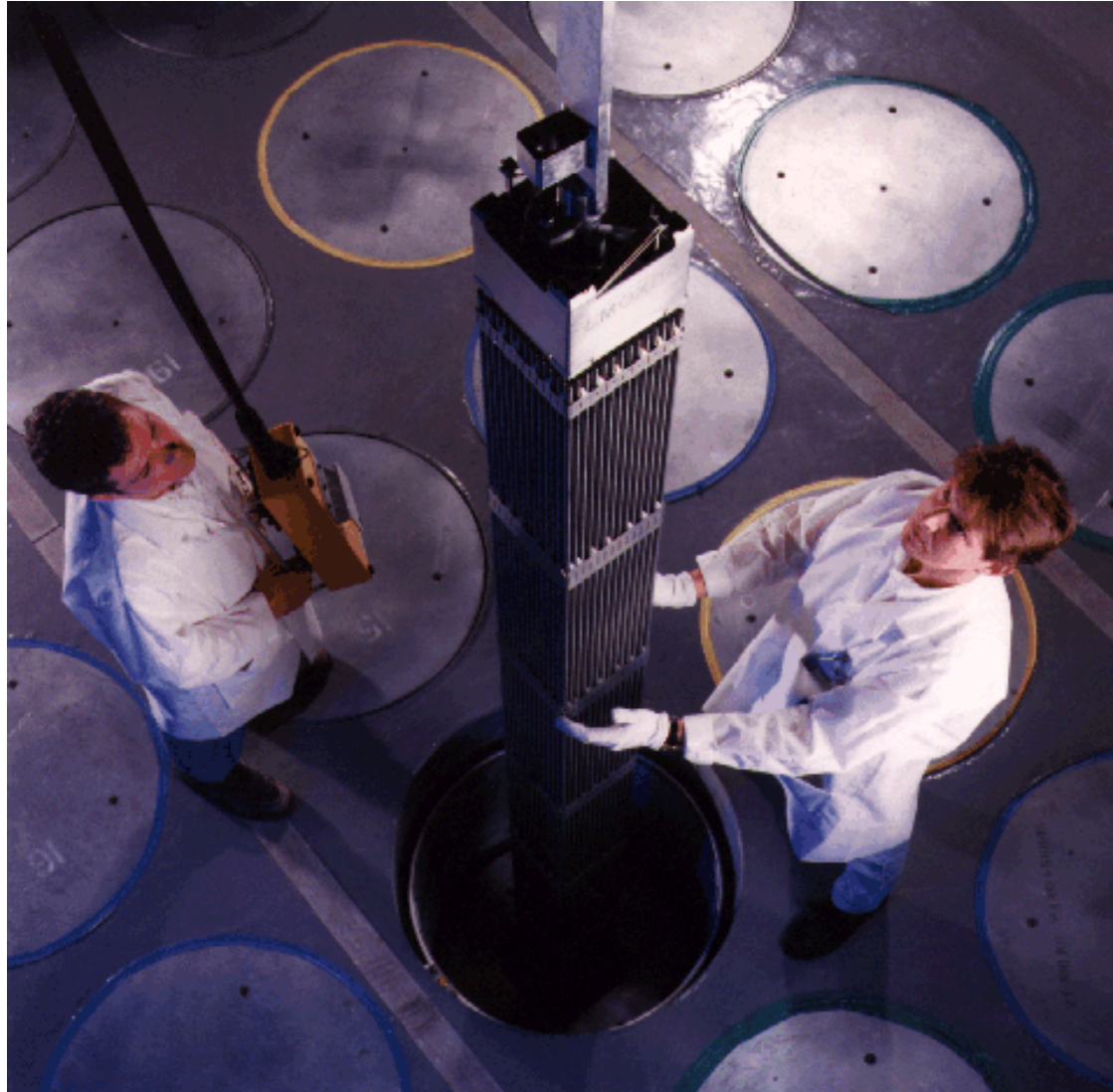
A pressurized water reactor fuel assembly
