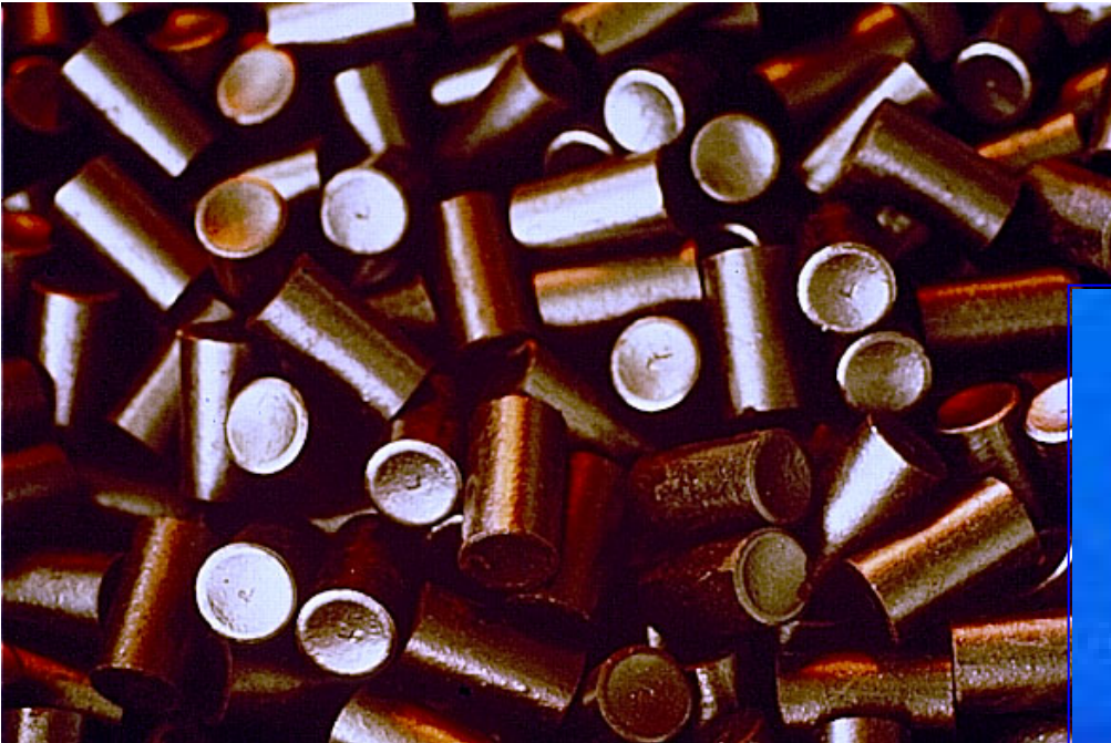
Uranium Oxide Ceramic Fuel Pellets
