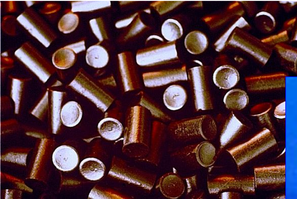
Uranium Oxide Ceramic Fuel Pellets
