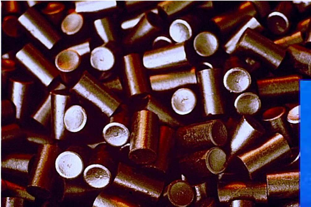
Uranium Oxide Ceramic Fuel Pellets
