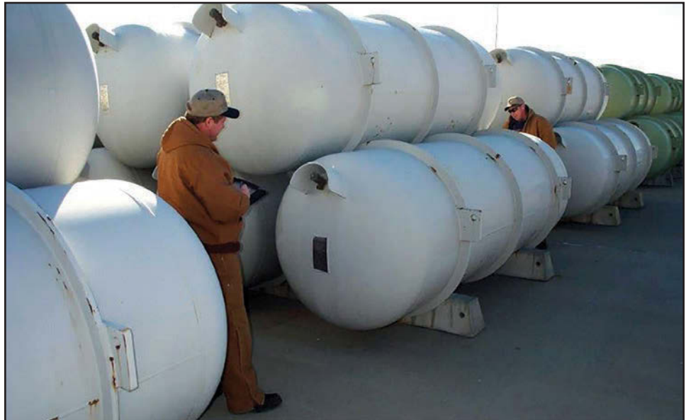
Workers inspect cylinders containing DUF_6 at a conversion facility at the DOE's Paducah site. (Photo: DOE)
