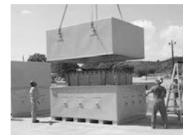
Split Cavity 23,500 lb MGW Reusable Overpack
