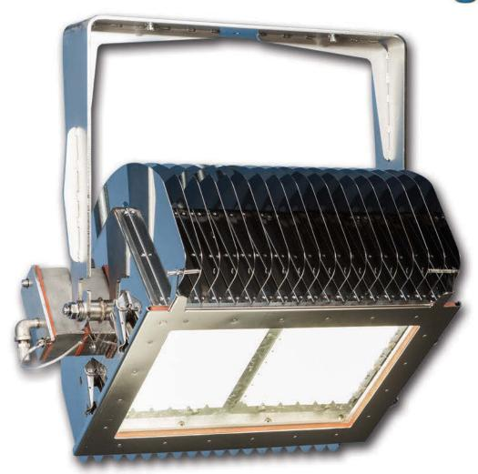
Our latest advancement in containment high bay lighting is the BIRNS Quantum-C™, providing powerful LED illumination for high ceiling and crane applications in a more compact footprint. Its ~109,000 hour lamp life minimizes maintenance and its 21,000 lumen brilliance enhances safety and productivity in a wide area. The seismically qualified BIRNS Quantum-C also features an exclusive breather system, so it withstands containment integrated leak rate testing at full pressure.
