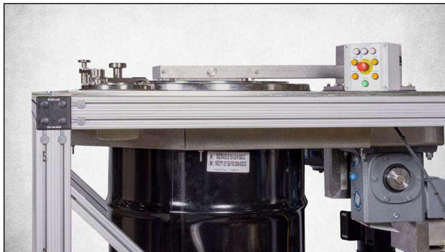
Electric motors raise and lower the drum, as well as rotate in and out of a locked position on the Alpha port.
